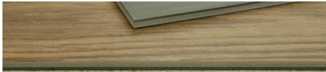
Close up view of specimen planks showing sectional profile.
