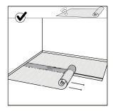
First lay the underlay across the breadth of the room and then gradually as you lay the planks.
