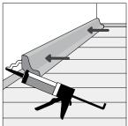
Install the skirting-board. Never attach the skirting-board to the floor. This method allows the floor to expand and contract under the skirting-board.
