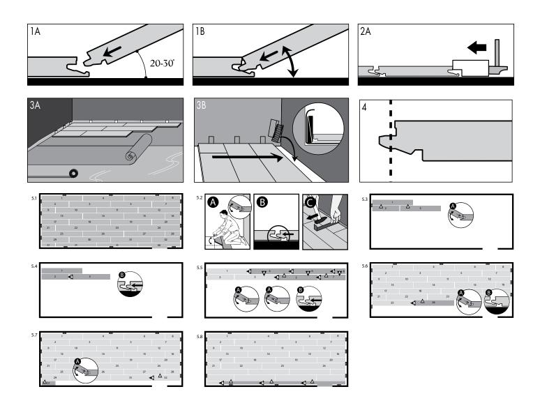
In the instance of knowingly or logically wet subfloors, or heated subfloors, always use 200uM builders plastic sheeting, overlapping joins by 300mm, taping joins with waterproof tape and turning up at walls or vertical fixtures. Door frames and architraves should be undercut prior to commencing installation using a scrap of flooring and a long, flexible hand saw(Fig 10). Undercut saws may be available from your local retailer and are specifically designed for this purpose.
