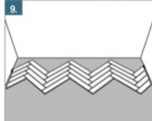
8. Continue with the B-panels Now work in the opposite direction, from the right to the left and install all the B-panels in the second row. Finish with a piece of panel cut to size (step5)
