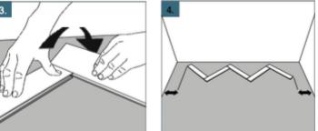
1. Getting started. Choose a wall to start at and begin installing at the left corner. Start with an A-panel and place it with its long side marking facing the left wall at an angle of 45°. Make sure that the distance between the left wall and the panel is less than the length of one panel.
