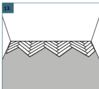
from the left corner. It is recommended to use glue to fix the smallest parts of the triangles into place by applying a small quantity of glue inside the groove.
