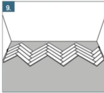
8. Continue with the B-panels Now work in the opposite direction, from the right to the left and install all the B-panels in the second row. Finish with a piece of panel cut to size (step 5)
